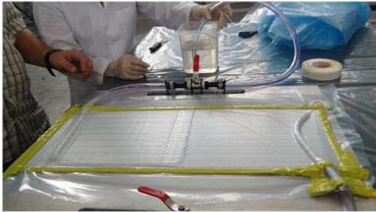
Manufacturing process: resin infusion
