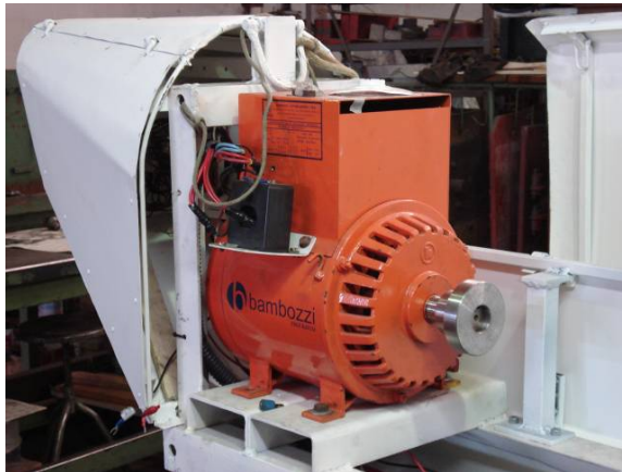
24 kW low-cost generator
