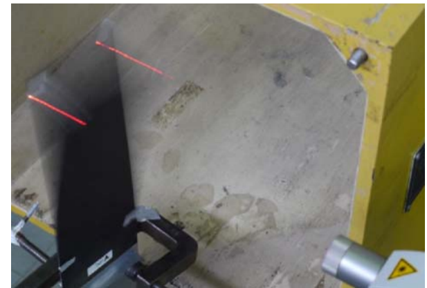
Aeroelastic measurement using laser vibrometer
