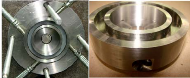
Rotational injectors improve fuel combustion efficiency
