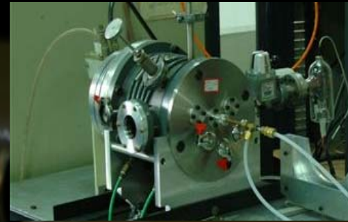
Reactor for thin film deposition for application in electronic and solar devices
