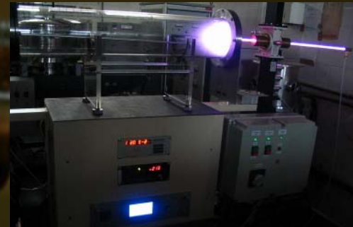
Surface treatment of rubber using plasma
